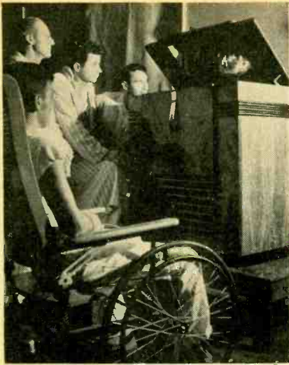
Television brings relaxation to war veterans. Set is RCA current model. Image is projected to mirror on lid.
